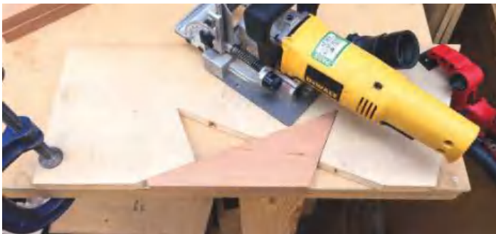
▲ Pic.15 Another jig was used to hold the components for cutting the biscuit slots in one side, followed by the other. I generally use too many rather than not enough biscuits
